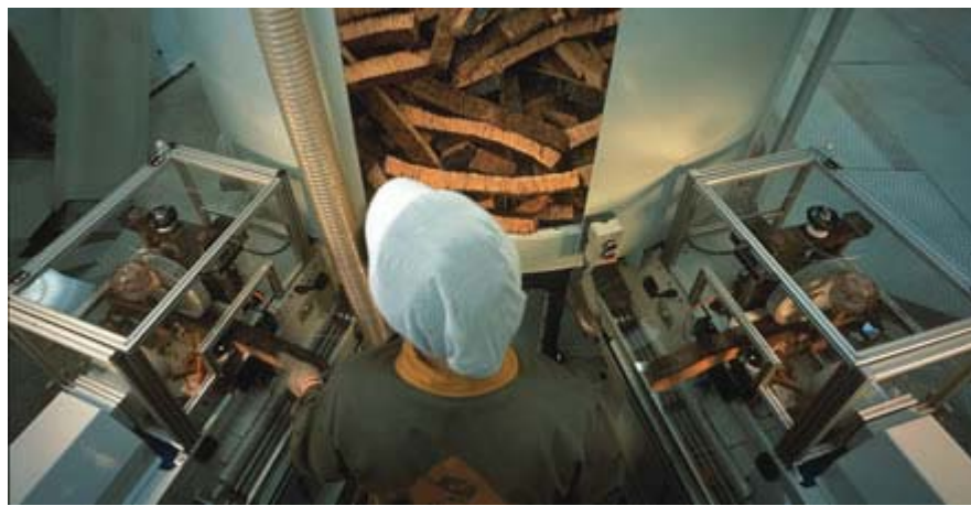
Strips of cork are fed into a cork-punching machine, with the grain running across the cork.
